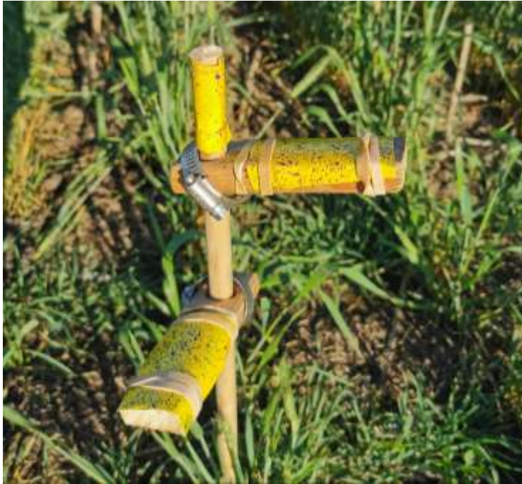
Figure 1. Stand with water sensitive paper to determine spray coverage received by wheat head, flag leaf and penultimate leaf.
